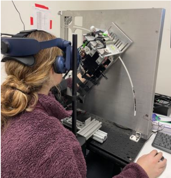
Virtual reality headset & arm secured in mobile robotic exoskeleton
